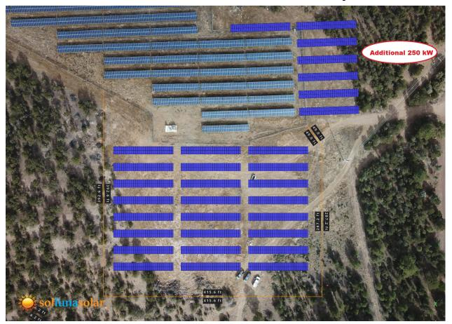
Phase IIa under construction has 1,440 Trina Solar panels w/2 Solar Edge 330 kW inverters
